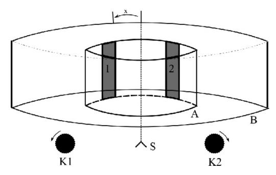
Figure 6: Two rotating hole experiment (side view). The two planar screens A and B are here replaced by cylinders. The position of each of the two holes 1 and 2 can be rotated with a knob ( $K_1$  and  $K_2$  respectively) and each knob can move the respective hole around the entire cylinder A.
